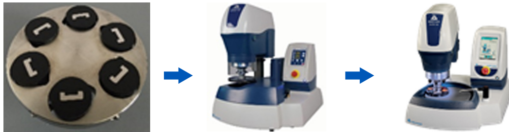
Figure 1 polishing process steps: clamping, grinding and polishing
