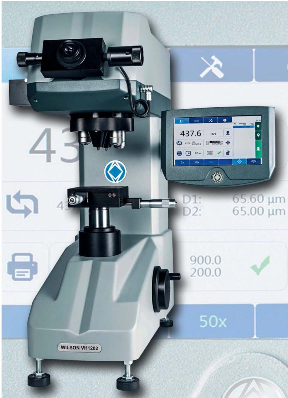
Wilson® VH1102 and VH1202 are two new universal hardness testers from Buehler – ITW Test & Measurement GmbH ([www.buehler.com](http://www.buehler.com)), offering a cost-efficient and reliable solution for Knoop and Vickers micro-hardness testing in accordance with ISO 6507, 9385 and 4546 or ASTM E384 and E92.
