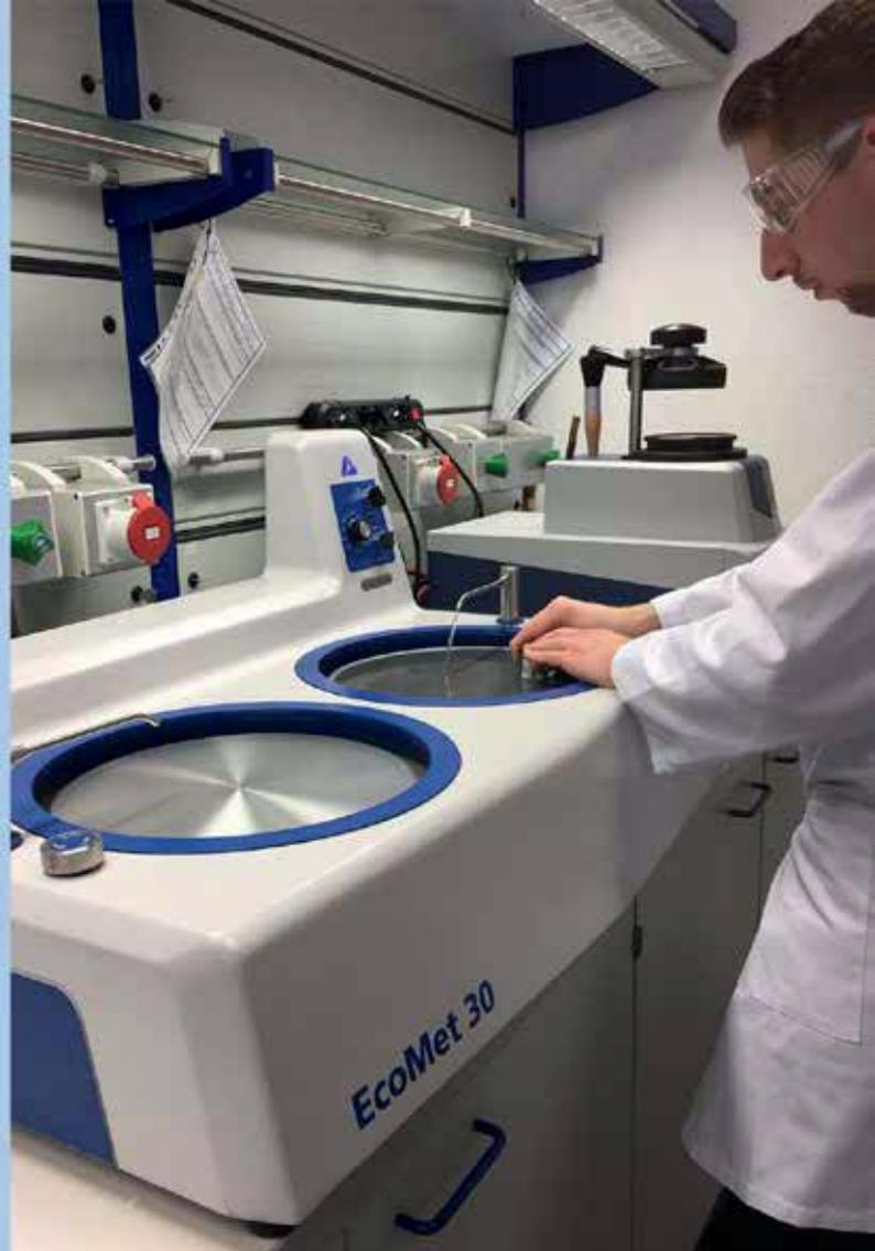
*The EcoMet 30 family of grinder-polishers from Buehler includes manual or semiautomatic, single or twin versions. These machines reduce labor and enhance productivity for routine sample preparation tasks – without compromising the consistency and quality of results. © ITW Test & Measurement GmbH*
